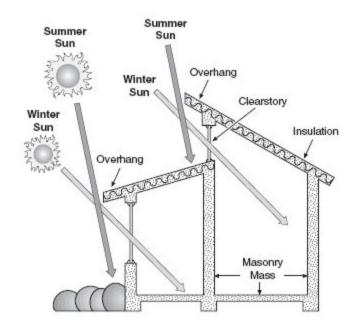
Figure 3.1: passive solar design
